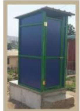
Biofil Alucobond Superstructure
