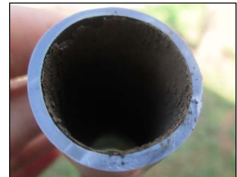
Dirt and biofilm inside a piece of pipe cut from hospital network.
